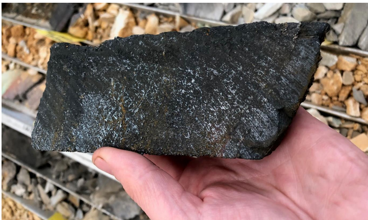
Chalocite-rich core sample from a drill hole in the Kamoia North Bonanza Zone. This sample graded 53% copper.
