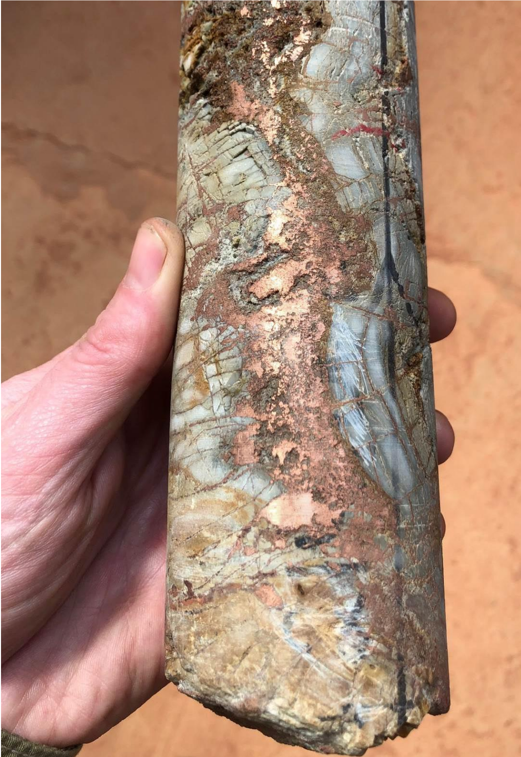
Figure 5: Core from hole DD1571 at a depth of 214 metres, showing disseminated chalcocite with a wide vein of native copper cutting through it in the breccia zone.
