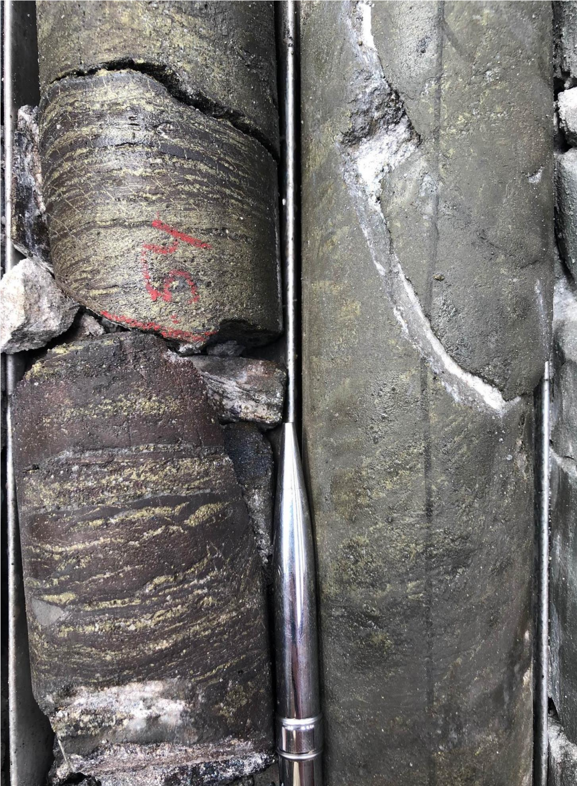
Figure 4: Core from hole DD1571 at a depth of 216 metres, showing massive bornite with traces of chalcopyrite.
