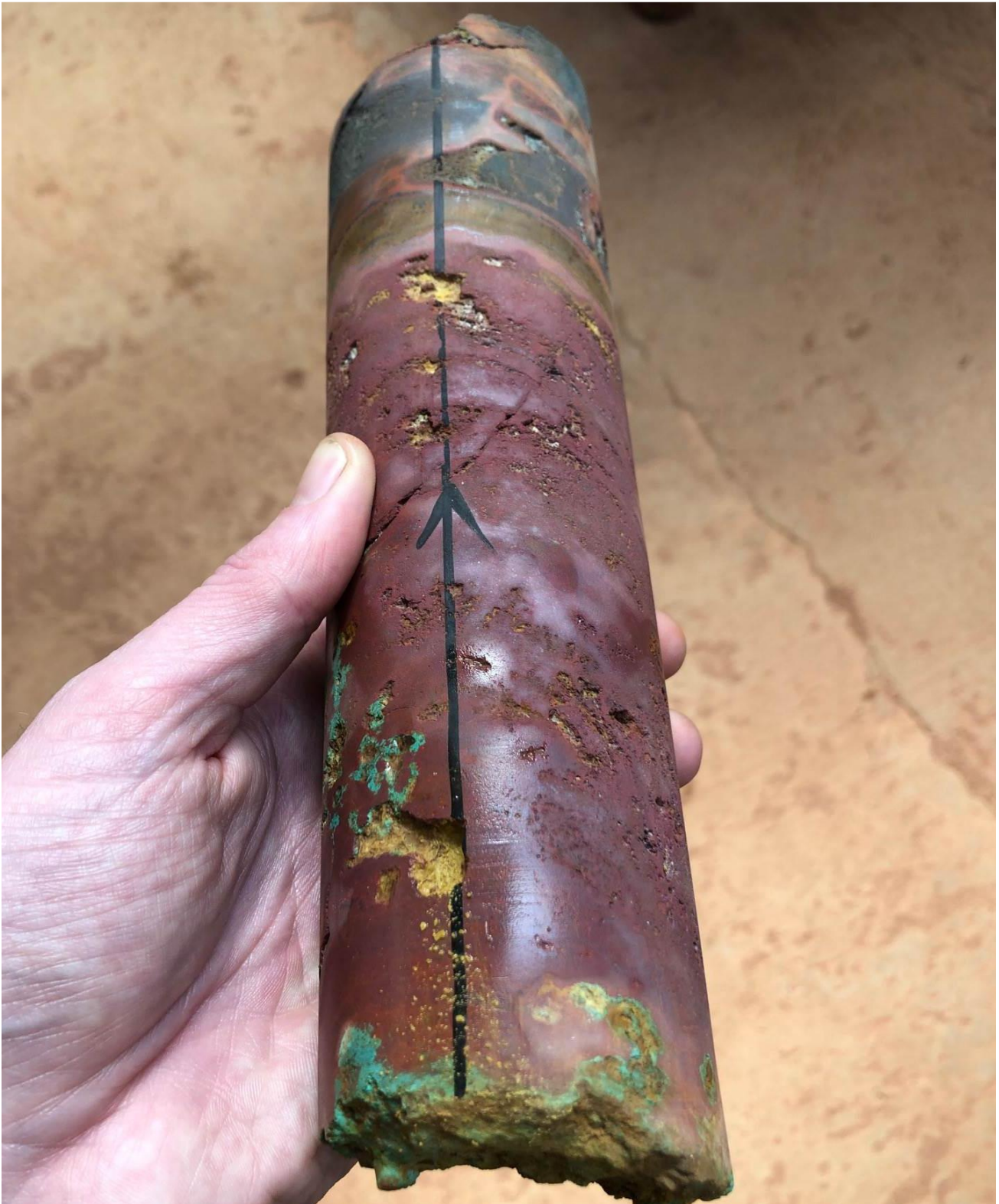
Figure 3: Core from hole DD1571 at a depth of 211.8 metres, showing almost all cuprite (cuprite, \text{Cu}_2\text{O} , is 88.82% copper by weight). Based on Niton readings, the average grade for the sample below is 37.7% copper.
