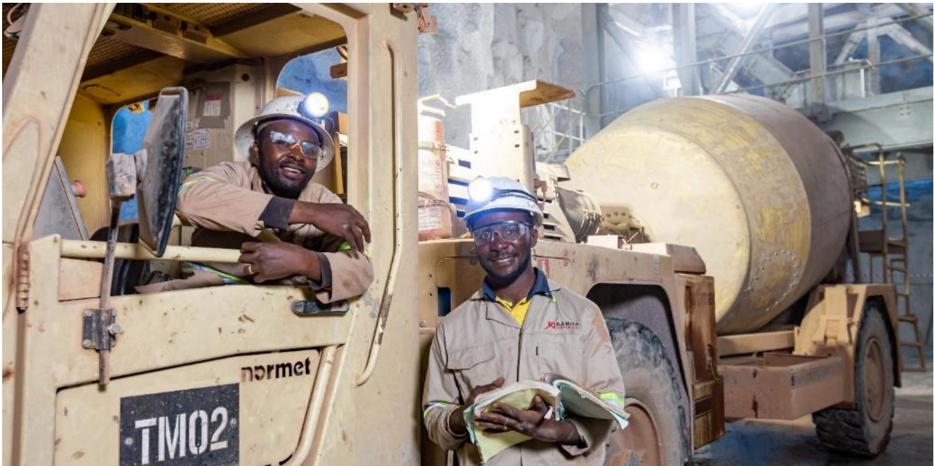
Kaimba Mwanza (left), Equipment Operator, and Jacques Muyumba, Technical Officer with AEL Mining Services, loading emulsion into one of the Normet Charmec explosives-charging machines.
