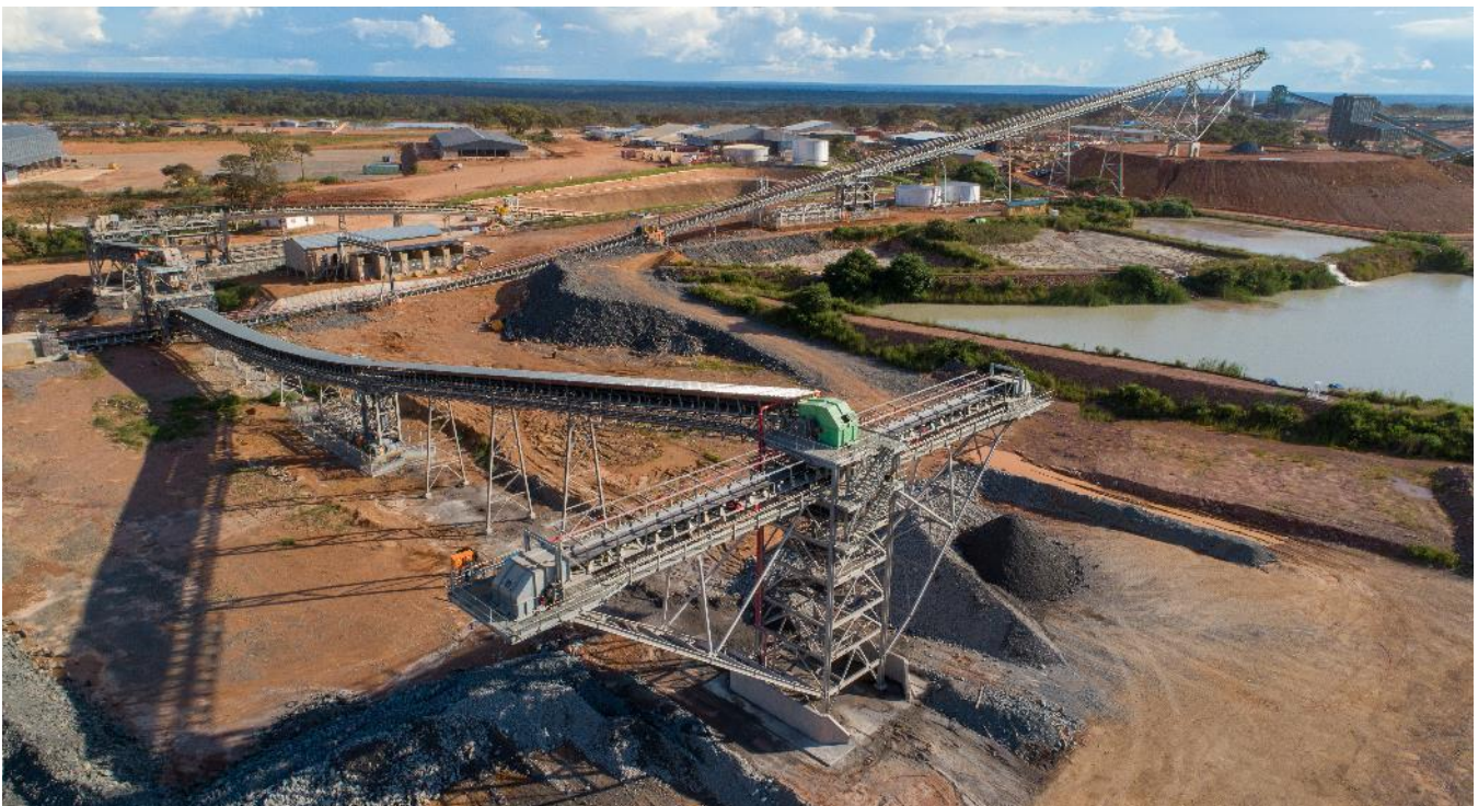
By-pass stockpile feed conveyor system, with the run-of-mine stockpile in the upper right corner.
