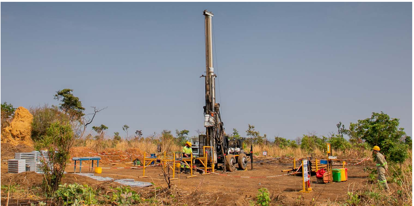
Figure 10: One of the drill rigs testing projected high-grade copper trends emanating from the northern part of the Kamoja-Kakula mining licence.
