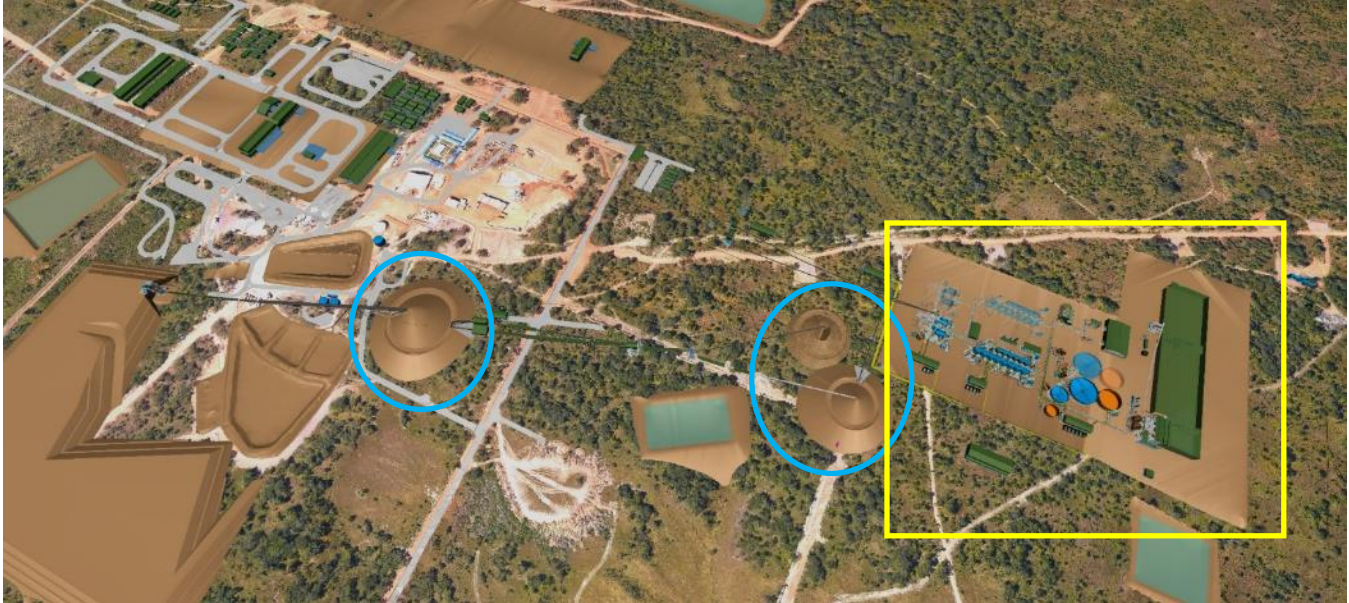
Figure 3: Kakula’s conceptual surface layout, showing the ore stockpiles (blue circles) and processing plant (yellow box).
