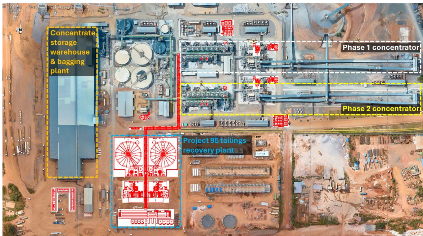
Photo: Infrastructure site plan of Phase 1 and 2 concentrators, showing new Project 95 equipment to be installed in red
