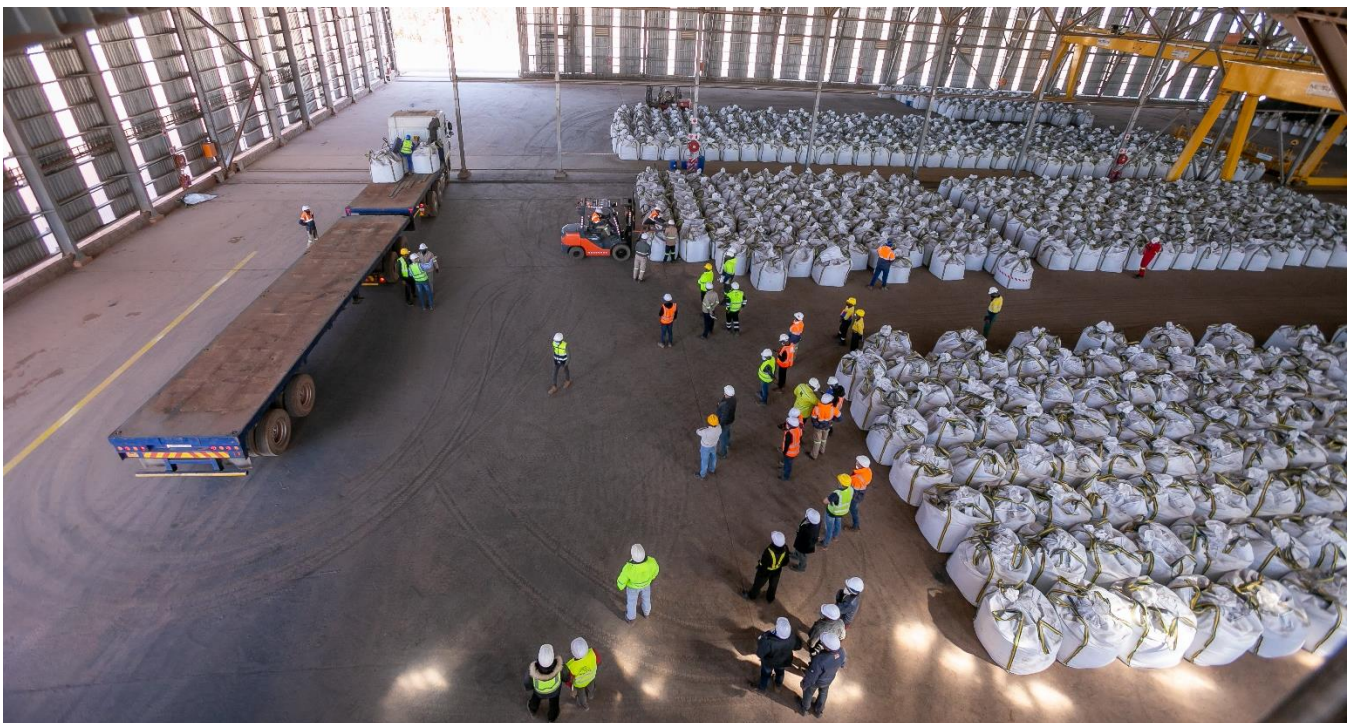
The first bags of Kamo-Kakula copper concentrate being loaded for export. Each bag contains approximately two tonnes of concentrate.
