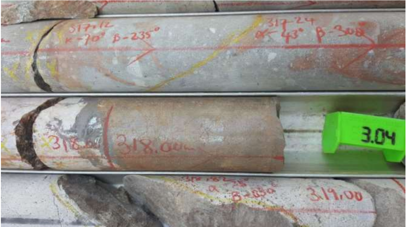
Figure 3. Intercept from DD1054, an in-fill hole near the centre of the Kakula Discovery, with massive chalcocite at a depth of 318 metres (chalcocite is approximately 80% copper by weight).
