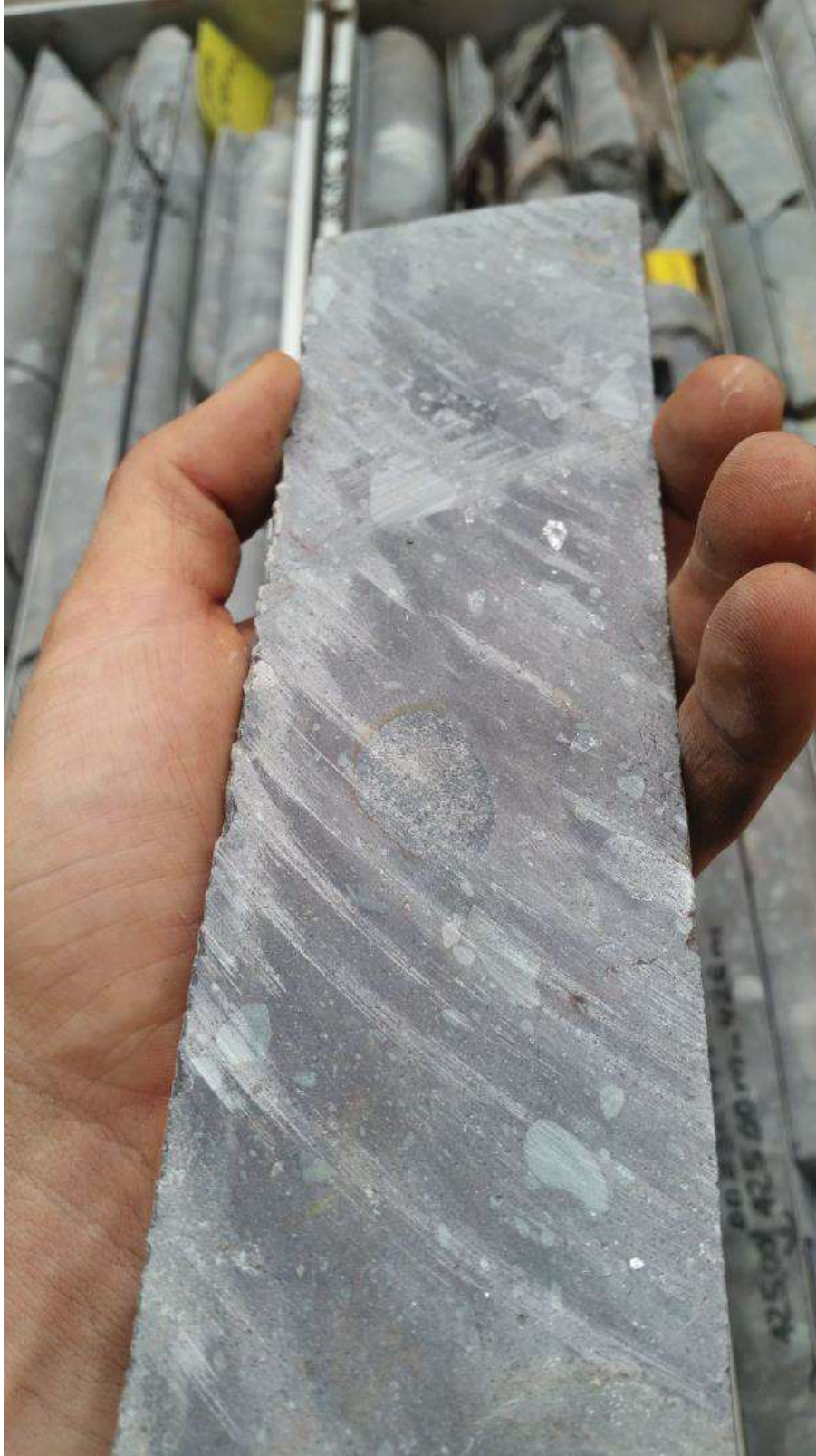
Figure 1. Drill core from DD1049 with disseminated chalcocite in diamictite at a depth of 422 metres (chalcocite is approximately 80% copper by weight).
