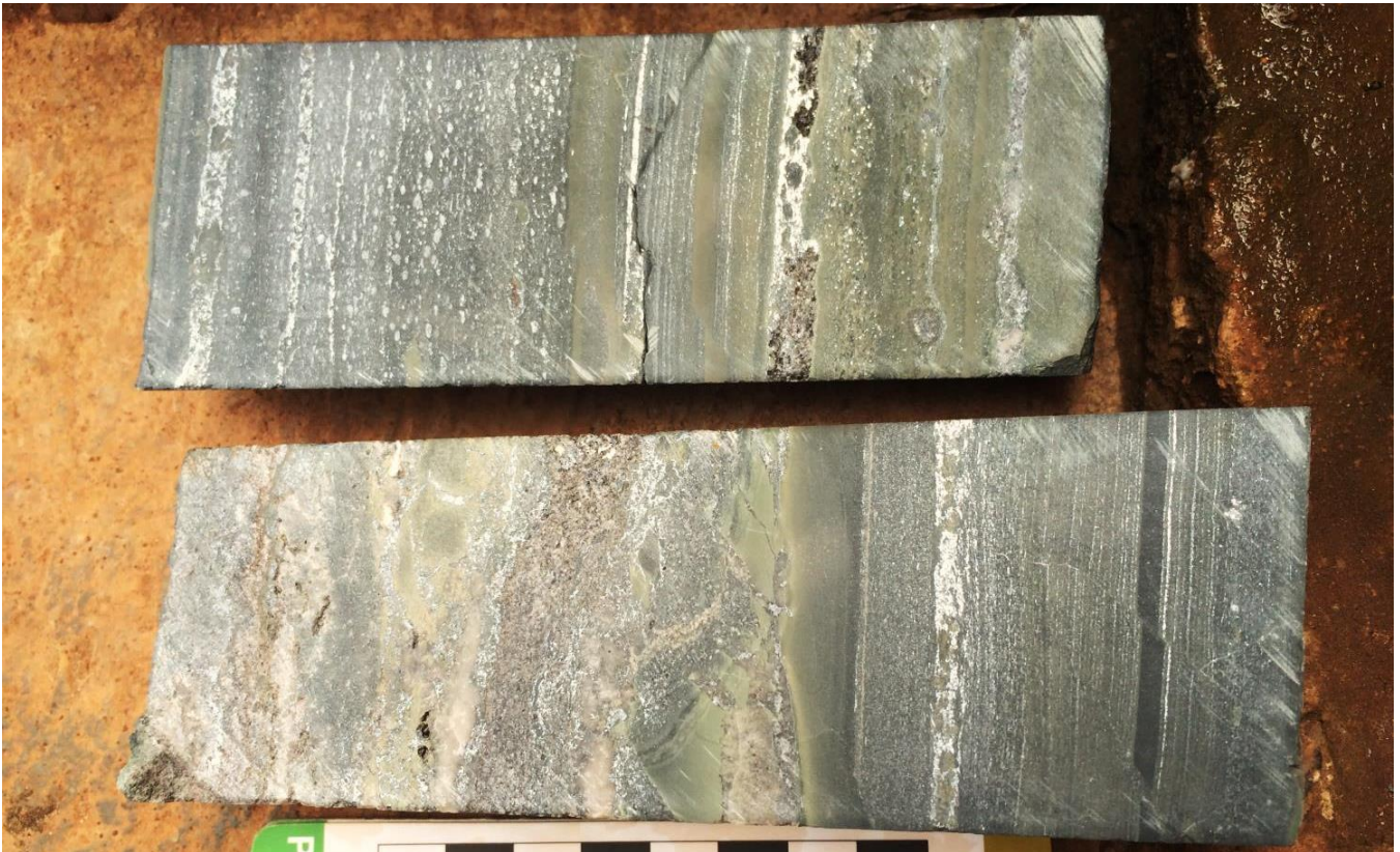
Figure 4: Finely disseminated chalcocite within bedded sandstone-siltstone. Sample grades at 15.00% copper from 375.45 metres to 376.00 metres in DKMC_DD996.
