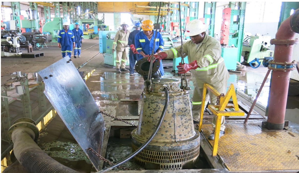
Figure 10: Testing 54-kilowatt Flygt pump in test pit.
