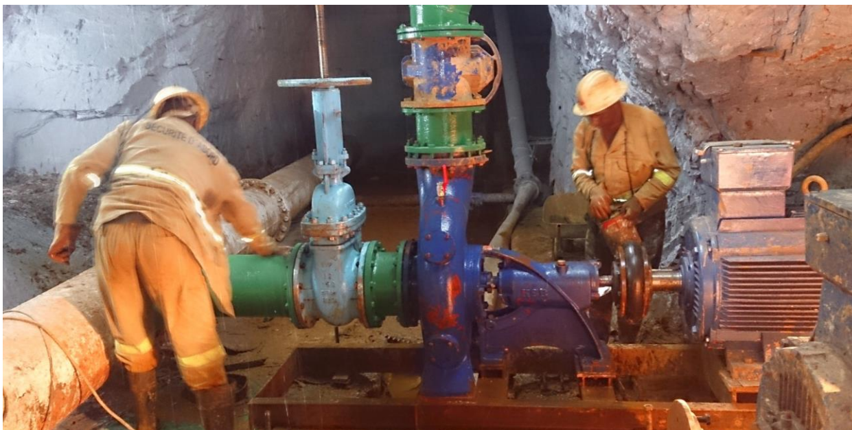
Figure 10: Testing 54-kilowatt Flygt pump in test pit.
