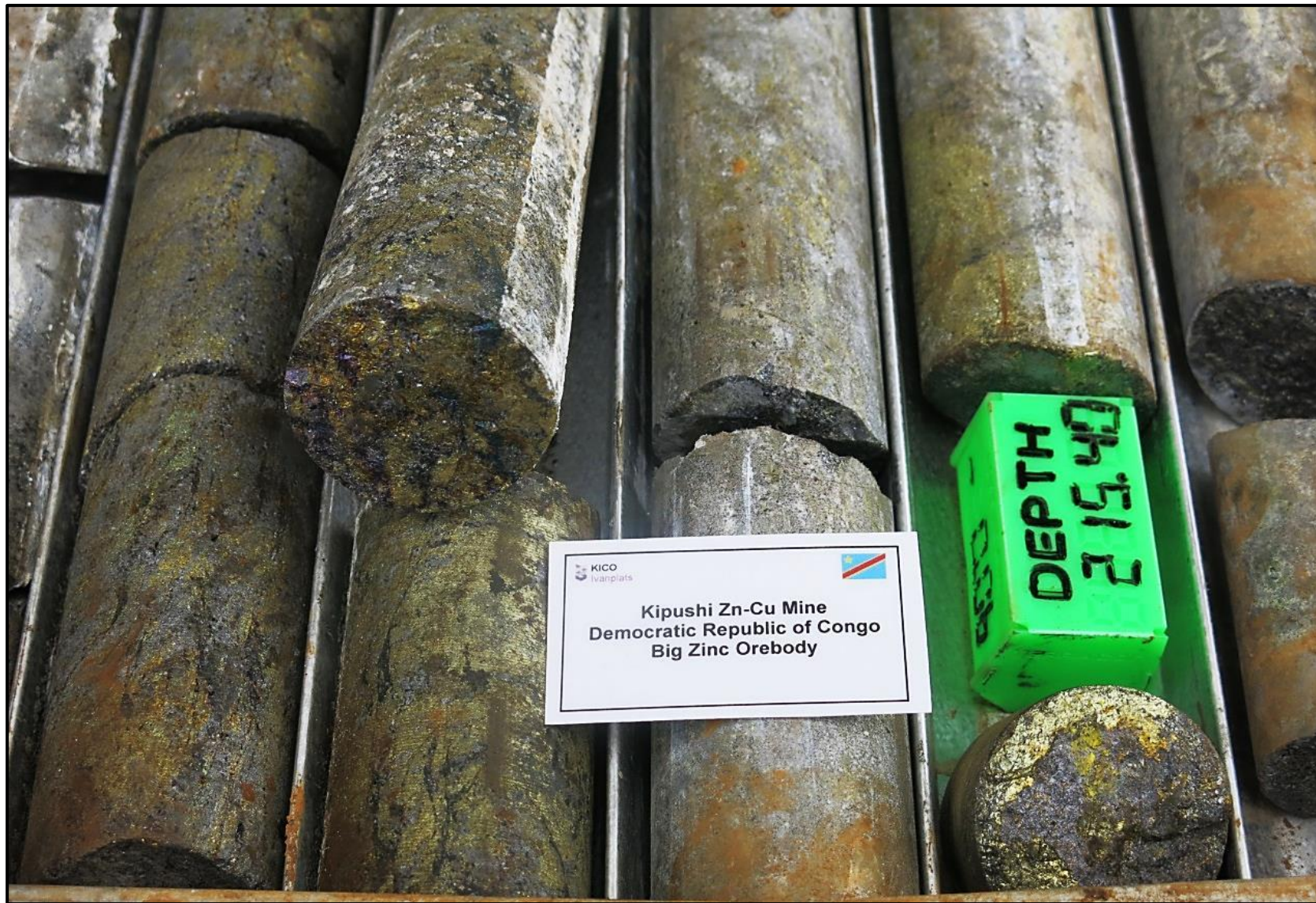
Figure 7: Hole KPU003 massive chalcopyrite-pyrite-sphalerite-galena intercept from depth of 207.8 to 215.4 metres (not true width).
