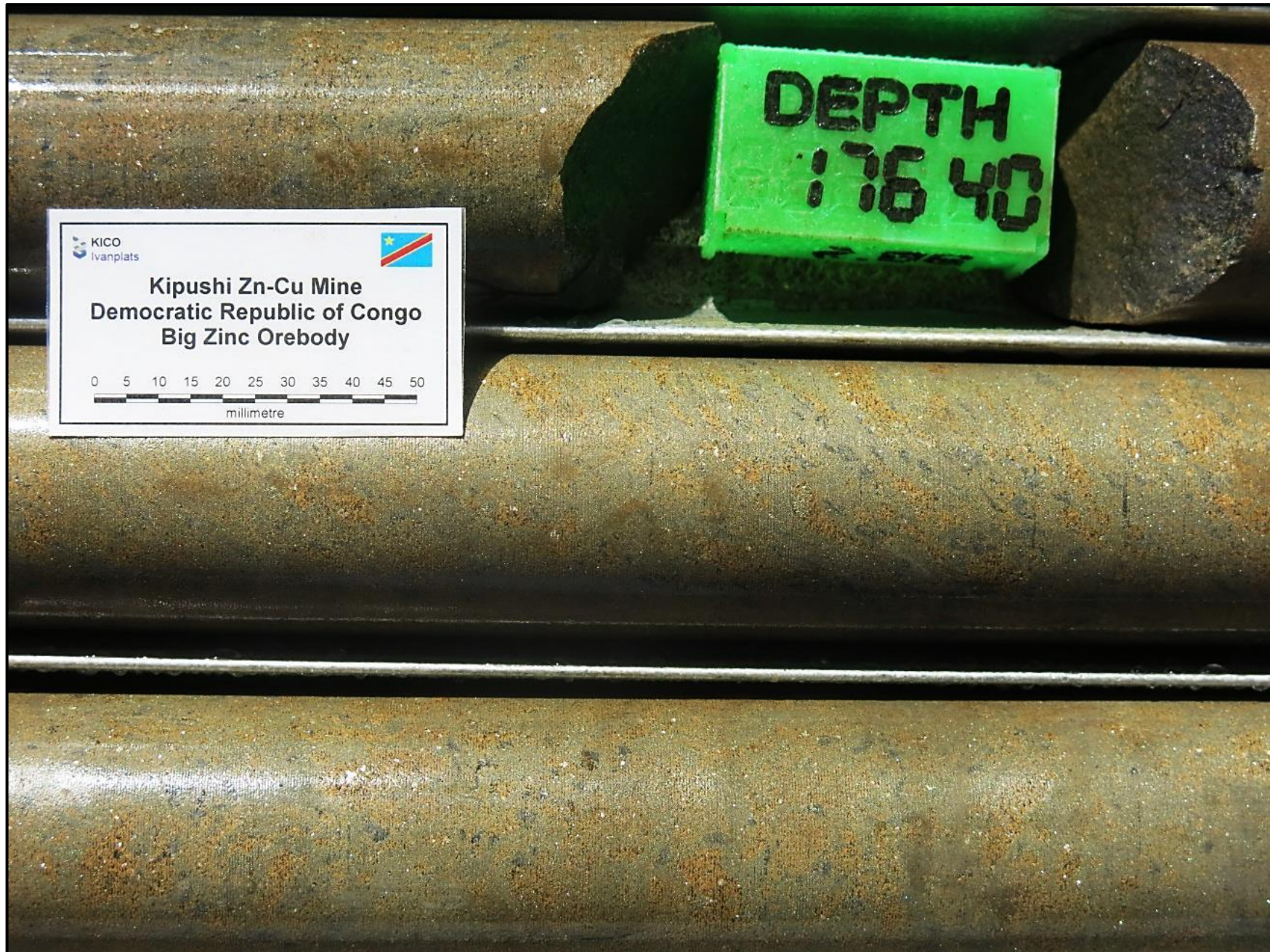
Figure 6: Core from Ivanhoe drill hole KPU003 showing massive orange sphalerite and pyrite.
