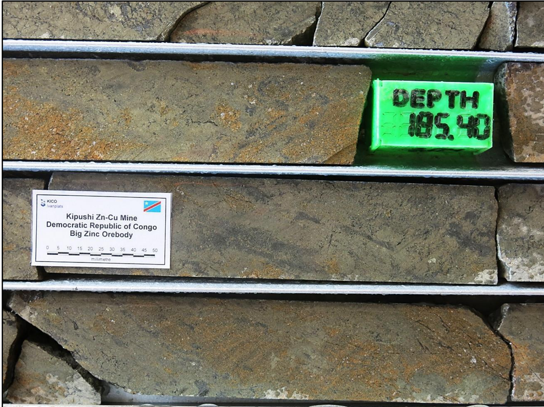
Figure 5: Core from Ivanhoe drill hole KPU001 showing massive red-brown sphalerite and pyrite.
