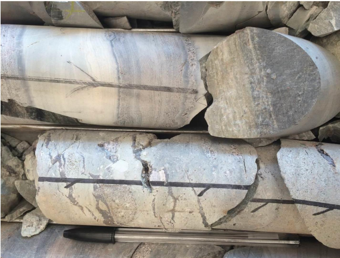
Figure 4. Intense chalcocite mineralization in siltstone layer at a depth of 511.6 metres in hole DD1045.
