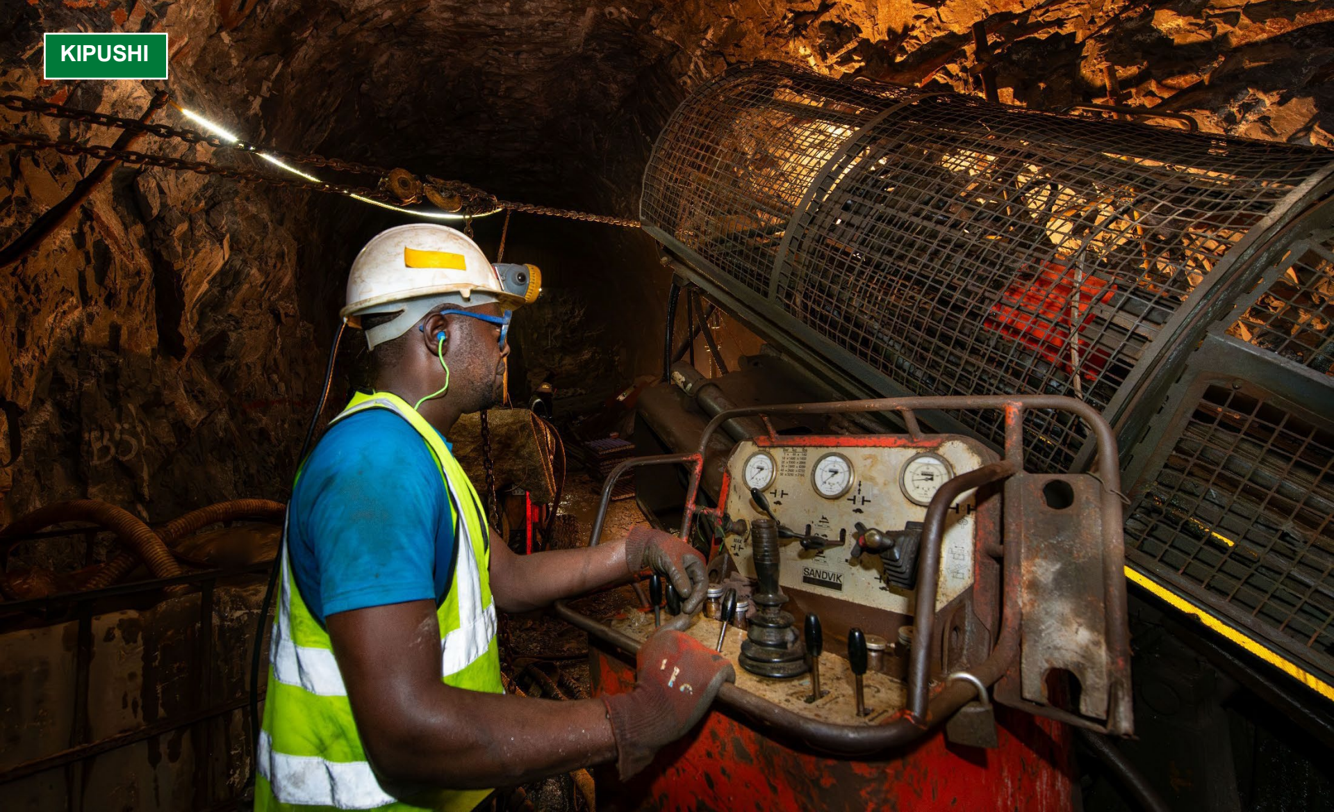
Moliere Kibamb, drill operator, at the controls of a diamond-drilling machine in Kipushi's underground workings.
