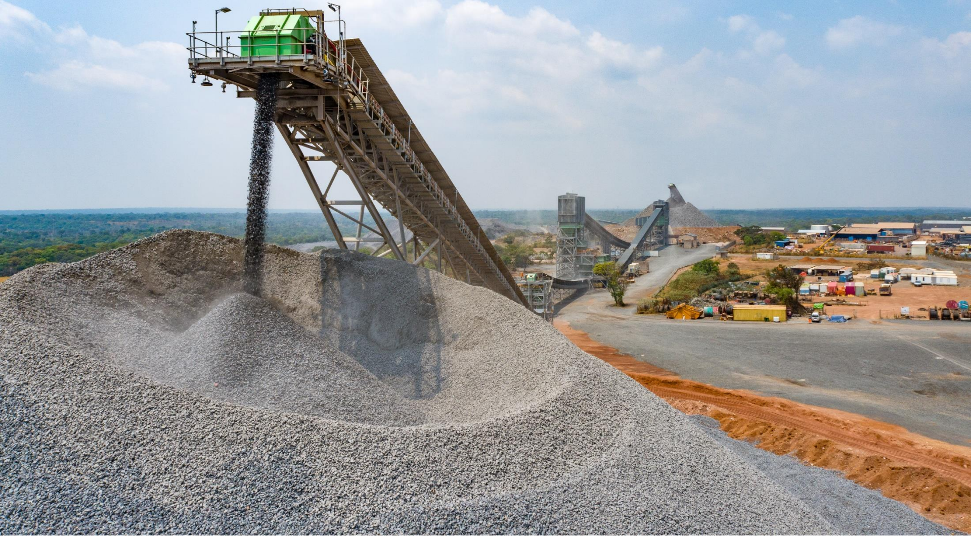
High Pressure Grinding Roll (HPGR) stockpile in the foreground and run-of-mine (ROM) stockpile in the background.
