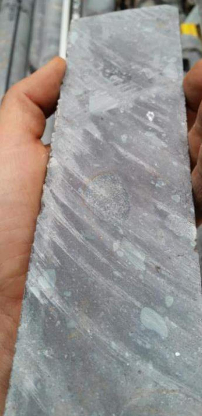
Core from Kakula drill hole DD1016, which intersected **8.75 metres** (true width) of **9.84% copper** at a 3.0% copper cut-off, beginning at a downhole depth of 362.0 metres.
