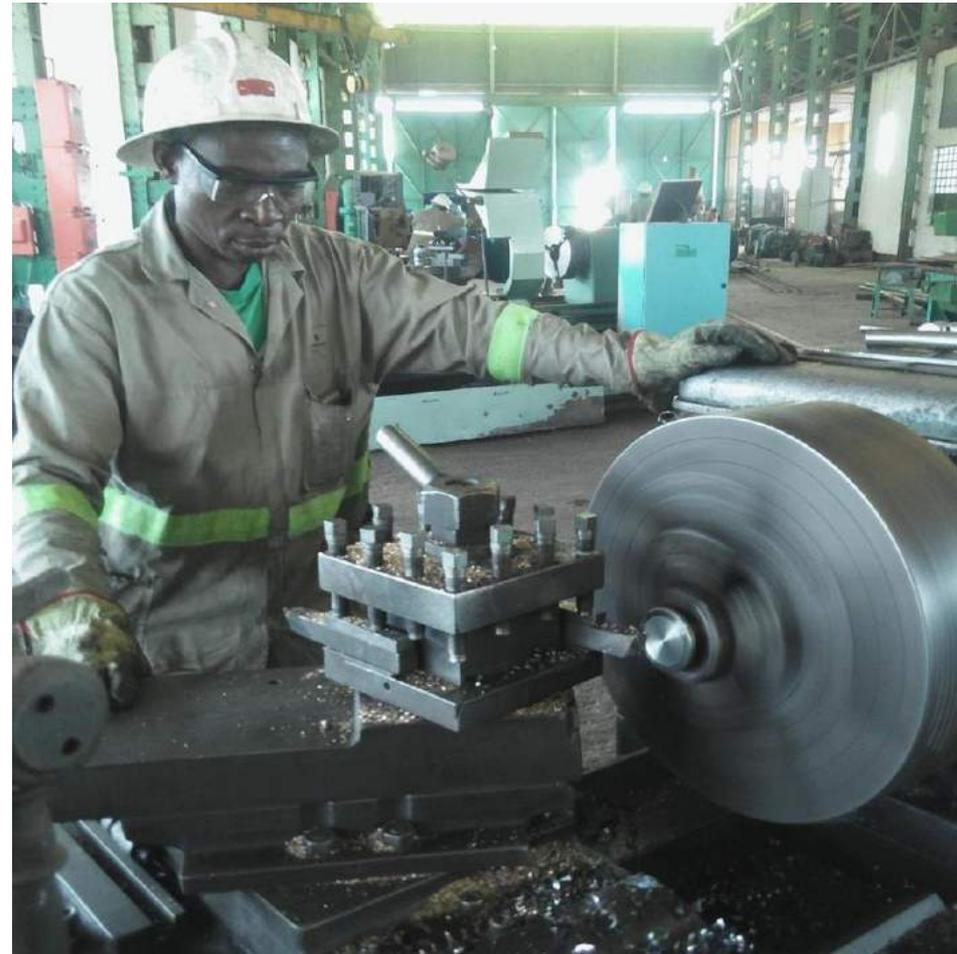
Machining flanges for plumbing installed at 1,240-metre-deep Shaft 5, which now has been upgraded and returned to working condition.
