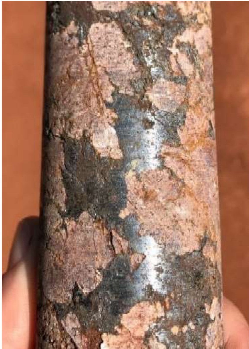
Figure 10: Massive chalcocite in a recent drill hole from Kakula West. Chalcocite is approximately 80% copper by weight.
